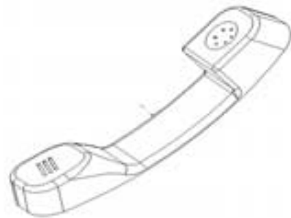
Figure 1. A telephone handset consists of three features: the ear-piece, the mouth-piece and the handle.
